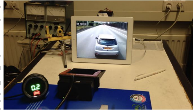
(a) Laser off, normal behavior of MobilEye C2-270
